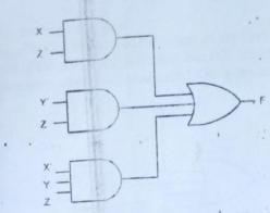
Introducing two successive inverters at the inputs of the OR gate results in the shown equivalent implementation. Since two successive inverters on the same line will not have an overall effect on the logic as it is shown before.
