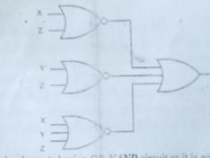
It can also be implemented using OR-NAND circuit as it is equivalent to NOR-OR circuit as shown in the figure. (see animation in authorware version)
